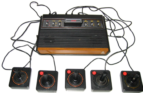
Figure 6. Chris Wren’s and Andrew Wilson’s multiuser UI, made out of old Atari joysticks.
