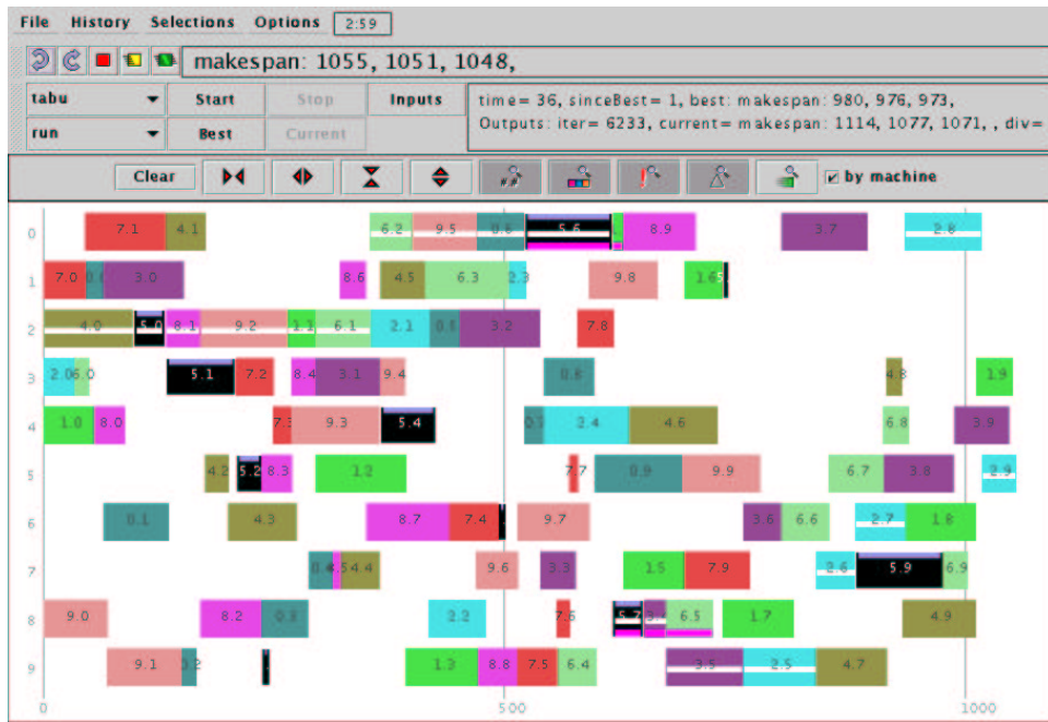
Figure 2: The Jobshop Application: the screenshot above shows our visualization in the mode for viewing operations by roster, where the background color of each operation indicates which job the operation is on. A white band in the middle of an operation indicates it is on the critical path, and a purple band on the bottom of an operation indicates its roster-position has changed from the previously displayed solution. Job number 5 has been selected by the user, by double-clicking on one of its operations, and so its operations are painted black
