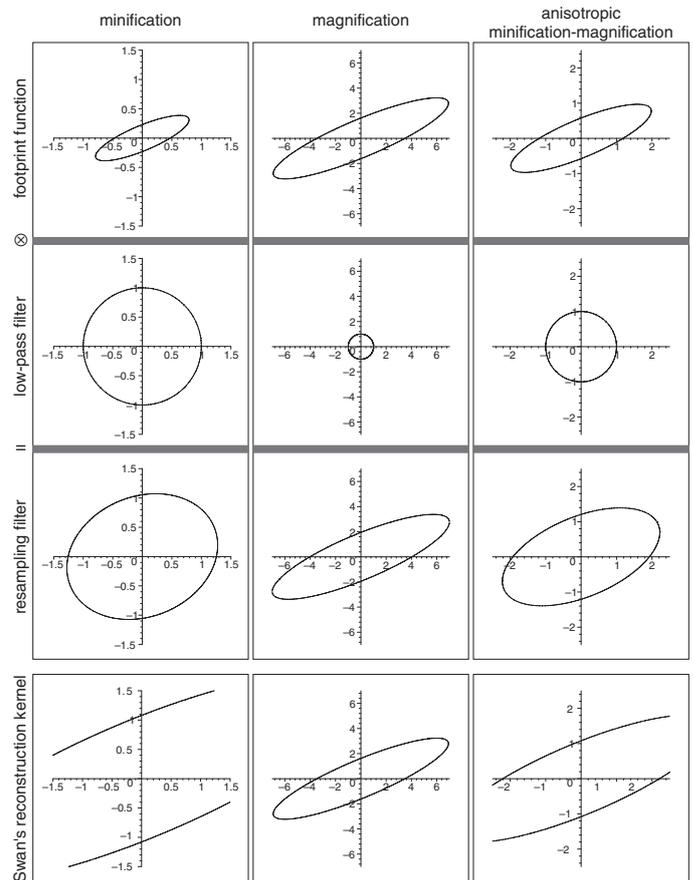
Fig. 13. Properties of the EWA resampling filter.
