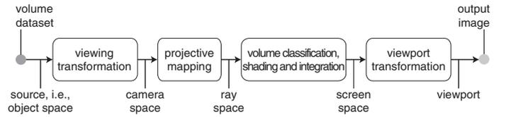
Fig. 4. The forward mapping volume rendering pipeline.
