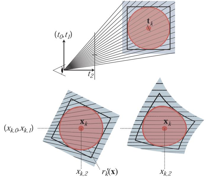
Fig. 9. Mapping a reconstruction kernel from camera to ray space. Top: camera space. Bottom: ray space. Left: local affine mapping. Right: exact mapping.
