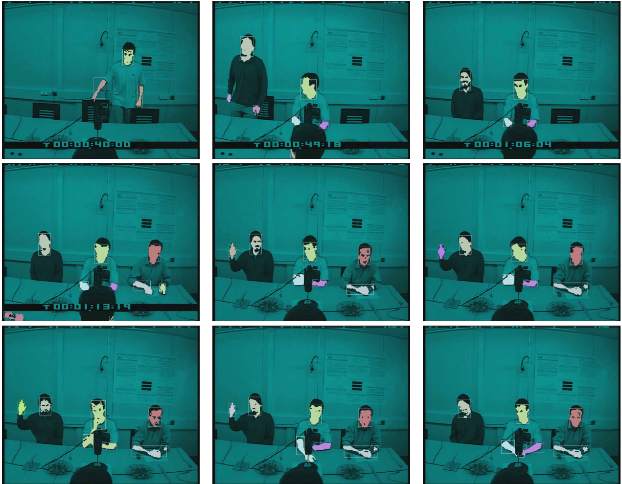
Figure 10: Tracking results for camera-1. Note that the heads are tracked accurately, i.e. each head has a unique color code.
