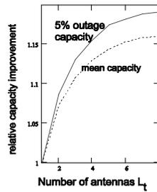
Fig. 4. Capacity increase of the 5% outage capacity and the ergodic capacity compared to  $L_t = 1$  when having several *active* antennas at the transmitter.  $N_t = 8$ ,  $N_r = 2$ ,  $SNR = 20dB$ .
