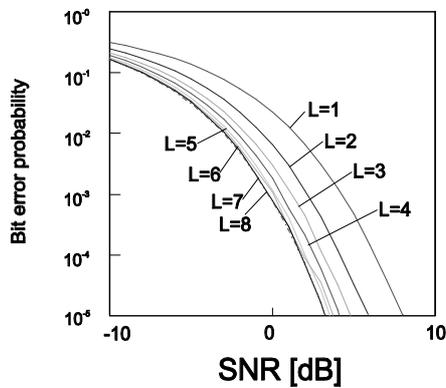
Fig. 5. BEP as a function of SNR for  $\pi/4$ -DQPSK as modulation format
