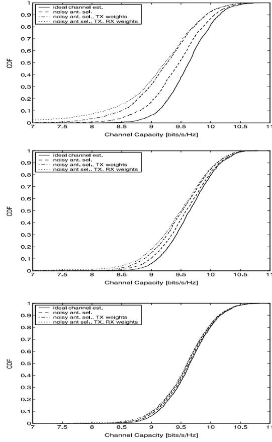
Fig. 8. Impact of errors in the estimation of transfer function matrix  $H$ . Cdf of the capacity for (i) ideal channel knowledge at TX and RX (solid), (ii) imperfect antenna selection, but perfect antenna weights (dashed), (iii) imperfect antenna weights at TX only (dotted), and (iv) imperfect antenna weights at TX and RX (dash-dotted). Top plot:  $SNR_{\text{pilot}} = 5$  dB, middle plot:  $SNR_{\text{pilot}} = 10$  dB, bottom plot  $SNR_{\text{pilot}} = 15$  dB.
