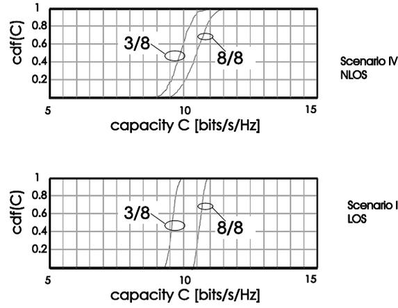
Fig. 9. Capacity of H-S/MRT system with  $L_t = 3$  and  $N_t = 8$  elements, and a MRT system with  $N_t = 8$  elements in a microcellular environment. See text for description of the scenarios.
