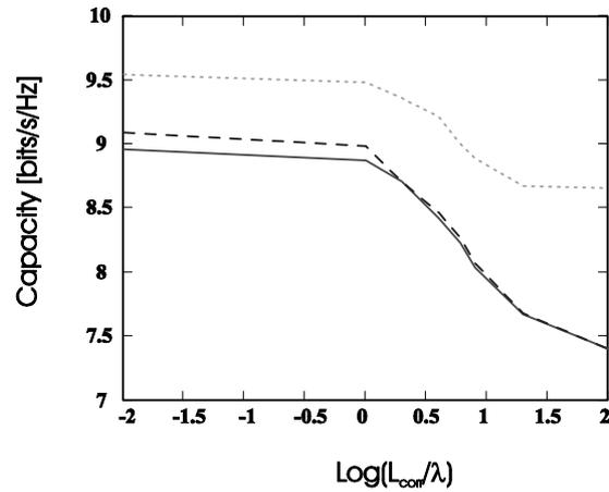
Fig. 6. 10% outage capacity of a system with 2 receiver antennas and H-S/MRT at the transmitter as a function of the antenna spacing. 3/8 system with optimum antenna selection (dashed), 3/8 system with antenna selection based on received power (solid) and 8/8 system (dotted). Correlation coefficient between signals at two antenna elements that are spaced  $d$  apart is  $\exp(-d/L_{\text{corr}})$ .
