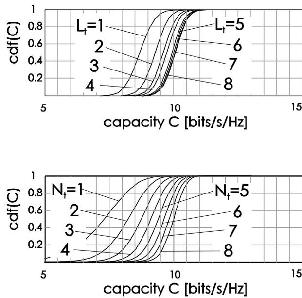
Fig. 2. Upper figure: Capacity of a system with H-S/MRT at the transmitter and MRC at the receiver for various values of  $L_t$  with  $N_t = 8$ ,  $N_r = 2$ ,  $SNR = 20$  dB. Lower figure: capacity of a system with MRT at transmitter and MRC at receiver for various values of  $N_t$  and  $N_r = 2$ ,  $SNR = 20$  dB.
