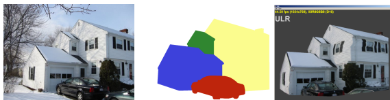
Figure 1: Left: Example input photograph. Middle: User labeling of image regions. Right: 3D model reconstructed from nine labeled images.
