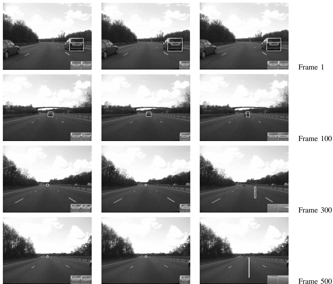
Fig. 4. The car sequence. Notice the fast scale change present in the video. Column 1: the tracking results obtained with an adaptive motion model and an adaptive appearance model ('adp'). Column 2: the tracking results obtained with an adaptive motion model but a fixed appearance model ('fa'). In this case, the corner shows the tracked region. Column 3: the tracking results obtained with an adaptive appearance model but a fixed motion model ('fm').
