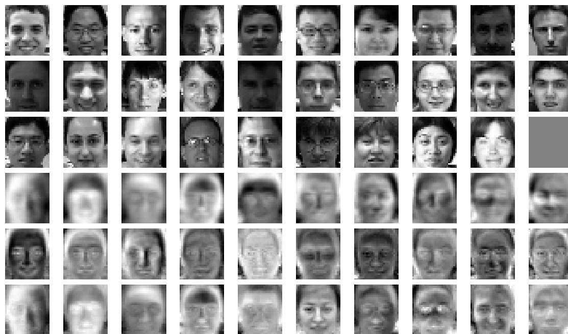
Fig. 10. Row 1-3: the gallery set with 29 subjects in frontal view. Rows 4, 5, and 6: the top 10 eigenvectors for the FFS, IPS, and EPS, respectively.
