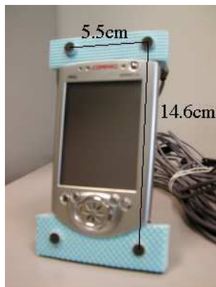
Fig. 3. A 4-microphone PDA mockup used to record the CMU WSJ PDA corpus.
