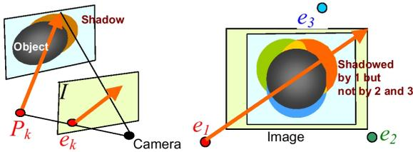
Figure 2: *Imaging geometry. Shadows of the gray object are created along the epipolar ray. We ensure that depth edges of all orientations create shadow in at least one image while the same shadowed points are lit in some other image.*
