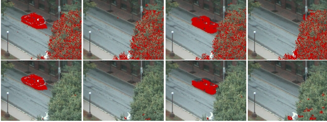
Figure 2: Background subtraction results. Top: unimodal approach. Bottom: DCT based method.
