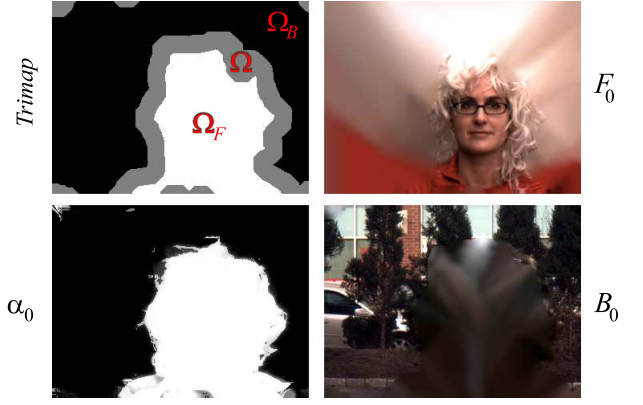
Figure 5: Clockwise from upper left: Trimap from defocus, foreground “outpainted” to fill space, background reconstructed from adjacent frames and inpainted, and matte via pinhole composition.
