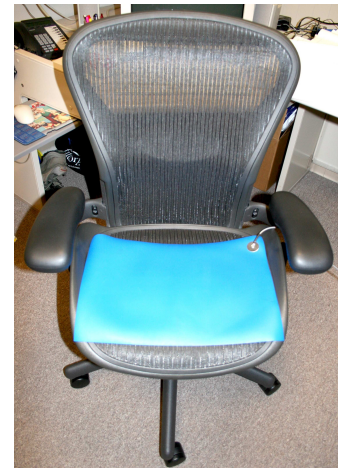
Figure 6: DT Controls receiver pad. There is one for each user.
