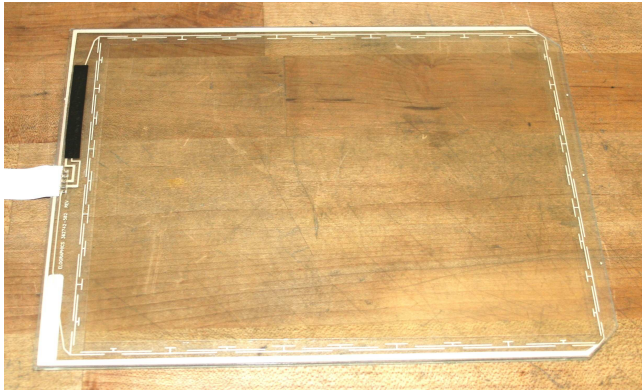
Figure 10: 5-wire, resistive touch screen.
