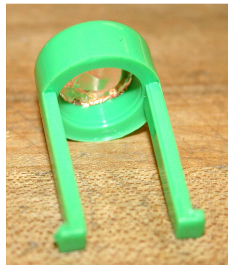
Figure 2: A push button which has been modified for DT Controls use. Note the copper foil on the inside top surface.
