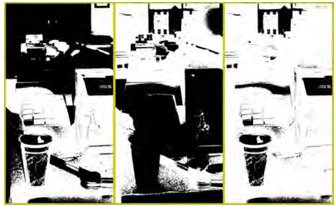
Figure 11: Optimal flash intensity and exposure ( P, E ) settings for the next picture. (Left) Pixels shown in white are captured with high SNR in the first two images (shown within the yellow and the orange boxes in Figure 8). (Middle) Pixels shown in white are captured with high SNR in the third image (shown within the green box in Figure 8). (Right) Pixels (in white) which are captured with high SNR using all three images. Note that almost all the pixels which are not captured with good SNR in the first two images (windows at the back, part of the table between the first and the second Macbeth chart) are captured with good SNR in the third image.
