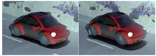
Figure 3: Vertical displacement by shifting the background and shadows. These two pictures are taken from the same camera position, so the car in both images is at the same location. Note (i) the change in position of the virtual shadows and (ii) the parallax for the edge between ground and backdrop with respect to the right headlight.
