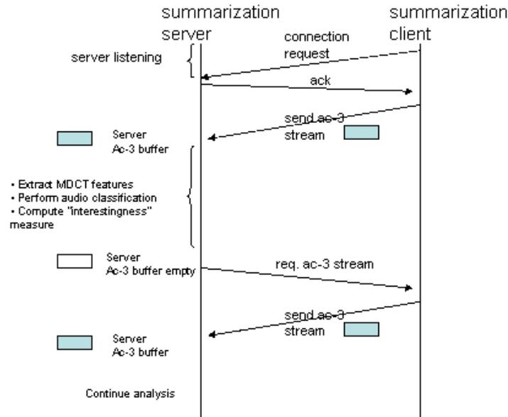
Figure 4: Timing diagram for a client-server implementation of summarization service
