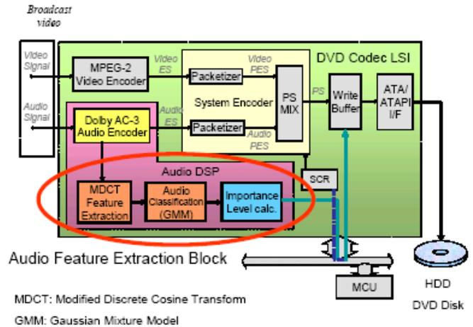
Figure 1: Architecture of a Summarization-Enabled DVD recorder
