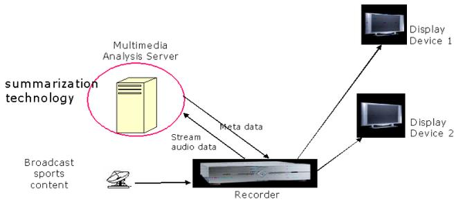
Figure 2: Architecture of a Summarization-Enabled Home Network
