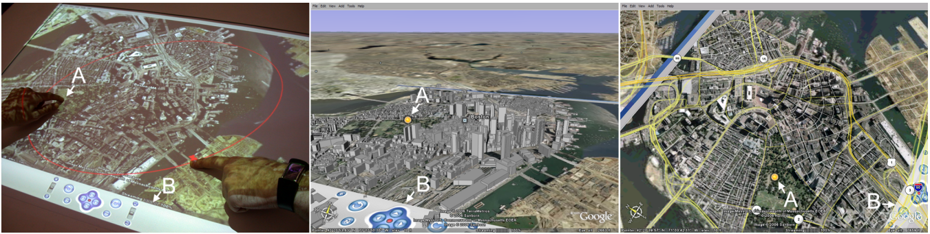
Figure 2: (note: the letters A & B are added to these images for clarity and are not part of the interface) All displays in the space focus on the same geospatial location from different views with different layers of information. The table ( left ) shows a bird's-eye-view, the first wall display ( center ) shows a 3/4 view with 3D buildings overlaid, and the second wall display ( right ) shows a wider view overlaid with roads. Dragging a proxy for the camera on the table controls the view of a wall display (red camera and control ring in the left image). Telepointers (A) on each wall display indicates the position touched on the table by the user in the left image. The navigation and title-bar displayed on the table are replicated on other displays (B) to help users understand the geometric relationship among views.
