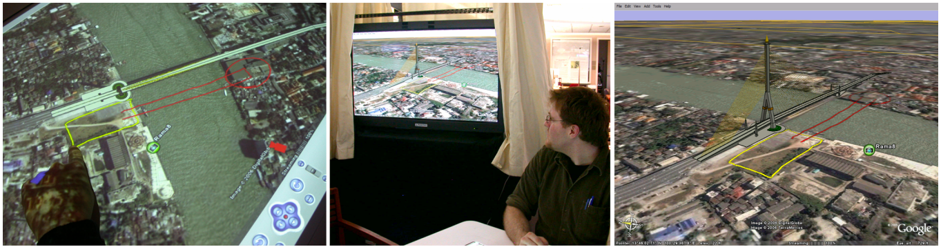
Figure 3: Multi-user annotations across different displays. (left) The strokes from each user around the table are drawn in different colors. (center) Annotations made on one display are geospatially registered so that they appear in the correct location on all machines. (right) Close-up of the wall display.
