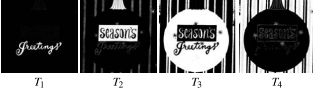
Figure 6: The blending weights computed from the “Season’s Greetings” dataset using SACLS with different settings of \lambda and \mu . Increasing values of \lambda force the algorithm to behave more like clustering, trading numerical accuracy for a more meaningful separation.
