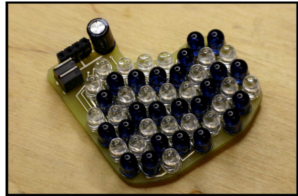
Figure 3. Light source of 24 red (clear) and 24 infrared (dark) high-output light emitting diodes.
