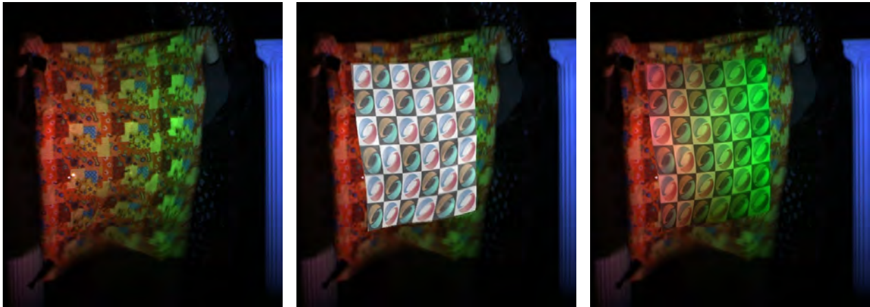
Figure 7: Synthetic texture with matched illumination. (Left) A cloth with 12 hidden tags. (Middle) Overlaying texture using the location and orientation of the tags. (Right) Texture modulated with incident illumination.
