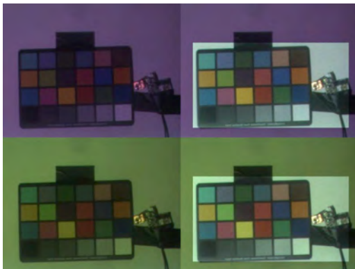
Figure 8: Computing intrinsic reflectance. (Left column) A color chart seen under purple and green illumination. The RGB sensor on the tag to the right senses the incident illumination spectrum. (Right column) We apply color correction to the center rectangle based on RGB sensor values.
