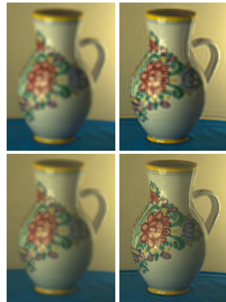
Figure 16: Comparison of traditional focus deblurring with a mask in the aperture. (Top) Captured blurred photo and the deblurred image for open aperture. (Bottom) Captured blurred photo and the deblurred image using the 7 \times 7 mask in the aperture.
