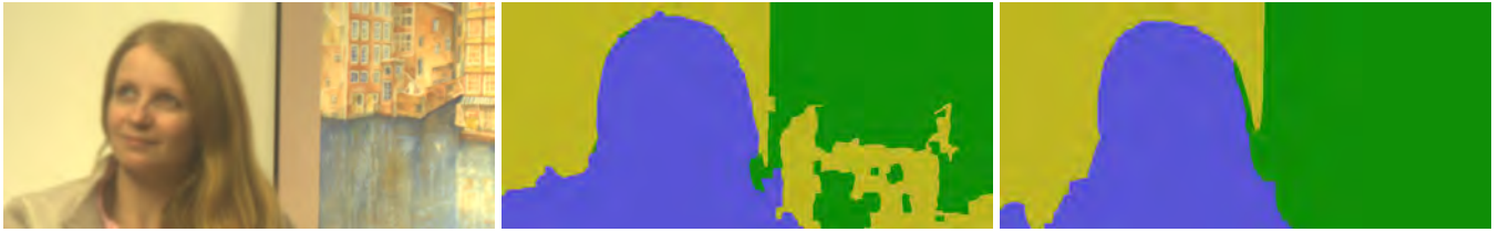
Figure 11: PSF estimation. (Left) Captured photo. (Middle) Initial crude segmentation of the scene based on the error maps indicate two dominant layers (person and painting) apart from homogeneous regions with scales 7 and 4 respectively. (Right) Final labeling for refocused image on the person by composing I_7 , reblurred I_4 and the captured blurred image.
