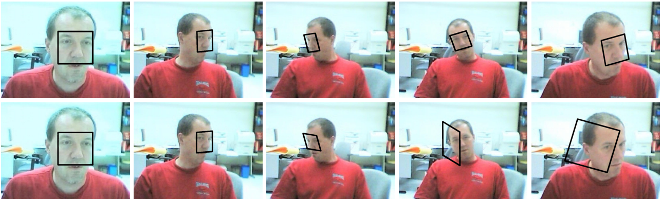
Figure 8. The effect of model update. The first row is with update. The second row is without update. The target has severe appearance variations due to illumination and pose change throughout the sequence. The sequence contains 324 frames.
