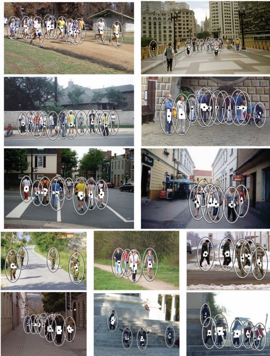
Fig. 16. Detection examples. The classifier is trained on the INRIA data set. White dots show all the detection results. Black dots are the modes generated by mean shift smoothing, and the ellipses are average detection window sizes. There are extremely few false positives and negatives.
