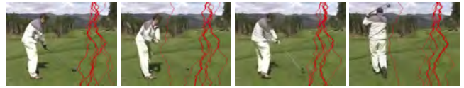
Figure 2: Seam carving on each video frame independently creates locally optimal seams that can be totally different over time. This creates a jittery resized video. In this example we show the first ten seams removed. A similar illustration is shown in the accompanied video.
