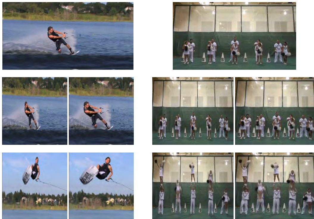
Figure 10: Examples of video retargeting. Top row, an original frame. In the following rows we show a rescaled frame on the left and a retargeted one on the right.
