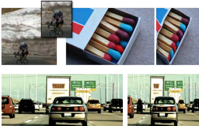
Figure 14: Cases where forward energy can fail. On the upper left, a snapshot from vertical resizing of a bicycle video sequence is shown, together with a zoom in on the bicycle rider. The bicycles are shrunk as the algorithm abstains from cutting the textured rocks. On the upper right, a grainy background texture is considered as important content, while the matchbox is distorted. On the second row, a frame from the highway video is shown with its corresponding frame from the retargeted video. Forward energy fails to achieve plausible result in this case due to the nature in which the camera and objects are moving. The actual result can be viewed in the accompanied video.
