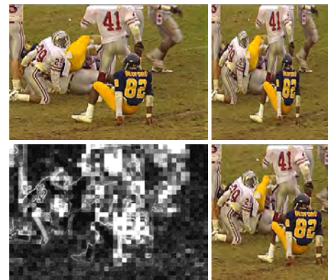
Figure 12: Retargeting using given energy (saliency) function. In the left column a frame from the football video is shown, and underneath is its saliency map. On the right column, on top is the rescaled frame, and at the bottom the retargeted frame.
