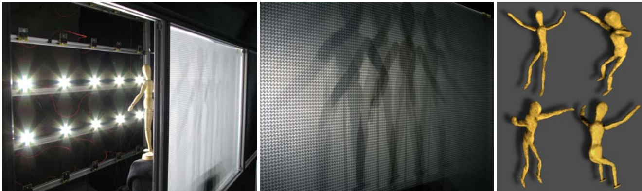
Figure 1: Our shield field camera allows instantaneous capture and reconstruction of the visual hull of 3D occluders using static illumination. (Left) The shield field camera, containing: an array of point lights, an object for reconstruction, and a large-format, mask-based light field camera. (Middle) Combined shadowgrams imaged on a diffusing screen after passing through a tiled-broadband attenuator. (Right) Four views of the visual hull reconstructed using only a single photograph captured by the proposed system.
