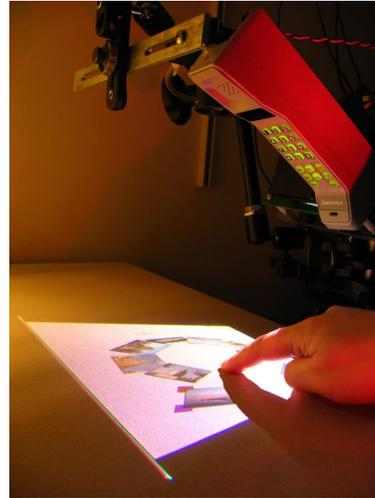
**Figure 1. A prototype cellphone-camera-projector device displaying a touch interface.**
