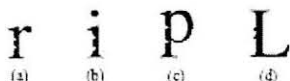
Fig. 1. Characters with different embedded symbols at 300% magnification. The distance between the notches or bumps encodes a symbol.
