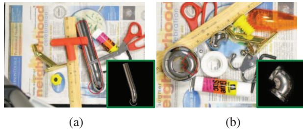
Figure 8. Failure cases for pose estimation approaches. (a) Since discriminative features are not visible on the end of pipe, estimated pose has large out of plane rotation error. (b) Specular reflections on a different object having similar shape lead to an incorrect match.
