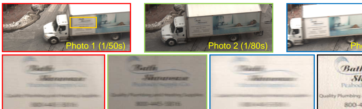
Figure 2: One can use widely available auto exposure bracketing (AEB) mode in consumer digital SLR to achieve PSF null-filling. Top row shows three photos of a moving truck captured using Canon Digital Rebel XT with AEB mode (exposures: 1/50, 1/80, and 1/30 sec). Bottom row shows the manually rectified blurred regions and the deblurred output. Notice that sharp features such as text are recovered in the deblurred image.
