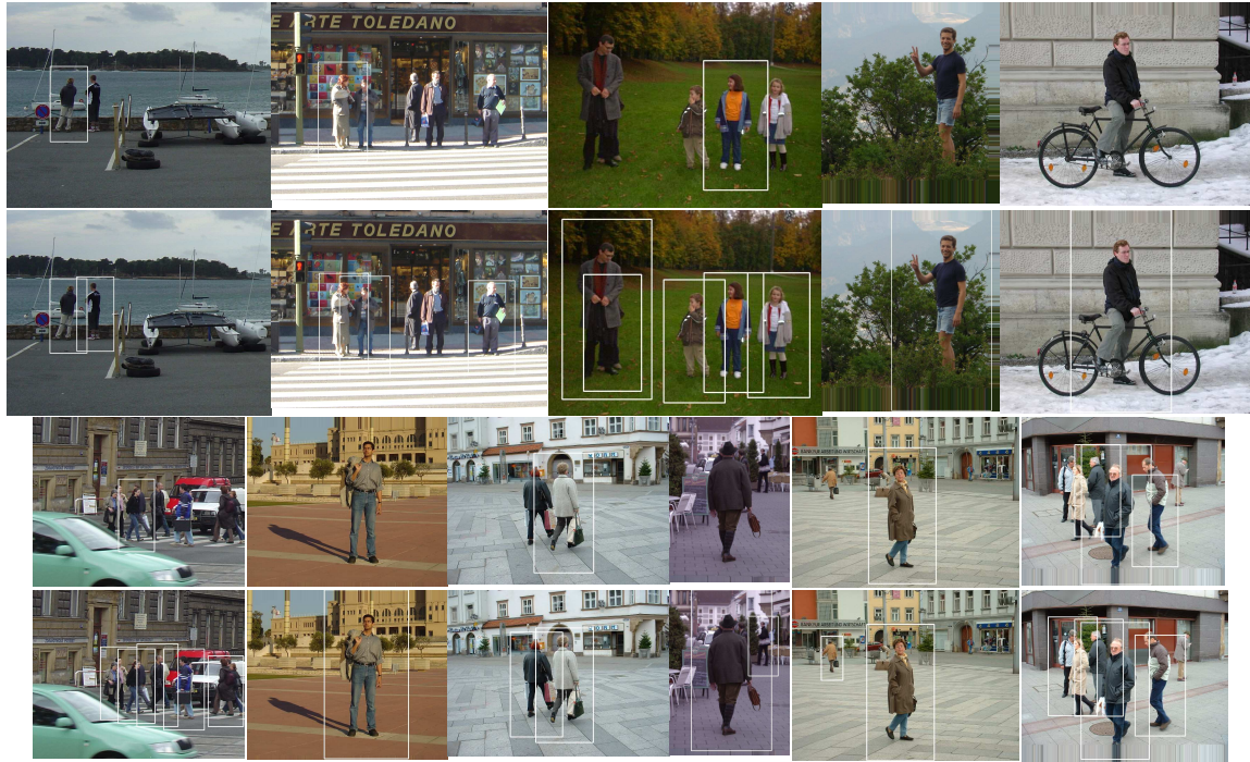
Fig. 6. Sample detections by the cascade boosted HOG features classifiers. The top image of every pair has the results from the Non-Def classifier (without d-features). The bottom image has the results with d-features with 2 refinement iterations and with a penalty term.
