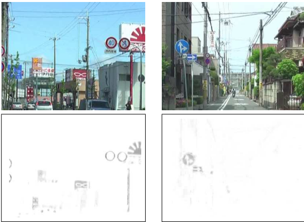
Fig. 2 The effect of applying the color filters (3) to the example RGB images (top row): red color filter (bottom-left), blue color filter (bottom-right). This figure is best viewed in color.
