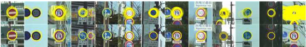
Fig. 8 Output of the Hough circle detector before (upper row) and after (lower row) applying the refinement procedure. The transparency of the detected circles in the upper row images correspond to their confidence expressed with the scaled number of votes picked from the Hough voting space.
