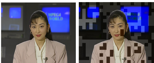
Fig. 6 The original image (left) and regions adopting RRU are marked with gray color (right)
