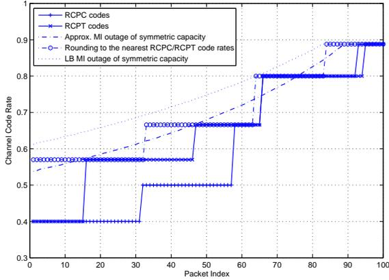
Fig. 7. Channel code rate profile of the baseline system at 18 dB
