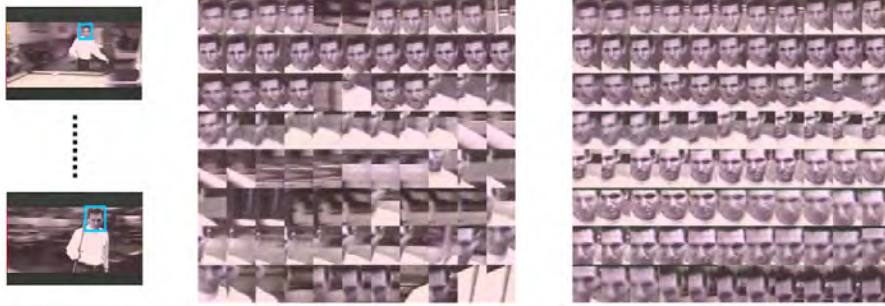
Fig. 6. Montages of the detection results (middle) without model update: detection rate is 47.7%, (right) with weighted mean based update mechanism on manifold: detection rate is 100%.
