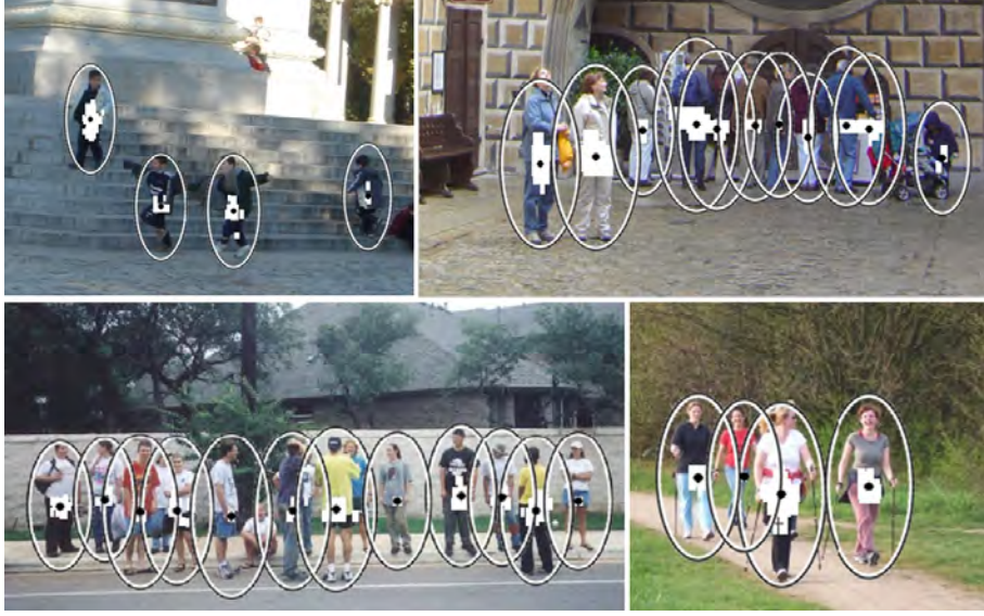
Fig. 14. Detection examples using cascade of LogitBoost classifiers on manifold. White dots show all the detection results. Black dots are the modes generated and the ellipses are average detection window sizes. There are extremely few false detections and misses.
