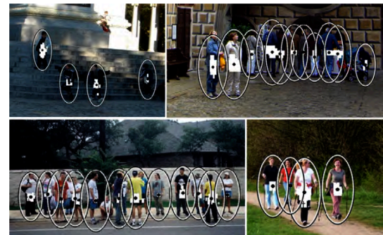
Fig. 14. Detection examples using cascade of LogitBoost classifiers on manifold. White dots show all the detection results. Black dots are the modes generated and the ellipses are average detection window sizes. There are extremely few false detections and misses.
