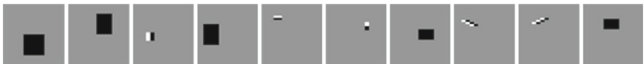
Fig. 13 10 best features selected by the SimBoost algorithm while training the 14-class road sign classifier using jointly the color-parametrized Haar wavelet filters and the histograms of oriented gradients. Both kinds of image descriptors are present
