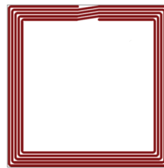
Figure 3. The geometry of resonant coil used in the analysis.
