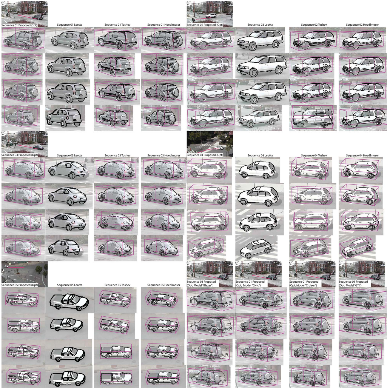
Figure 10. Classification and pose estimation results. One sequence is represented by four columns where each column shows results using different methods. The upper leftmost image of each sequence shows its first frame and our optimized projected track. The last four columns on the lower right show a variety of wrong model projected onto the image plane. See text for details.
