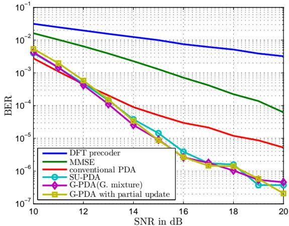
Fig. 6. Block size  $N = 16$ , QPSK modulation, measured channel, ten iterations. Remark: all algorithms yield the same performance with DFT precoder. All other plots correspond to identity precoder.
