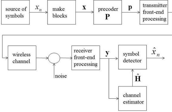
Fig. 1. Block diagram of a SISO communication system with block transmission and detection.
