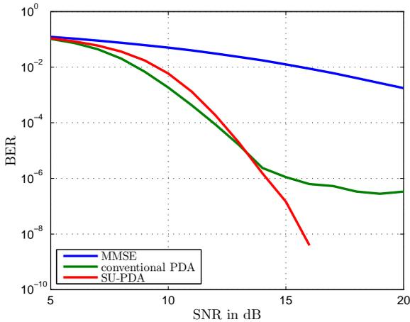
Fig. 4. Block size  $N = 64$ , QPSK modulation, DFT precoder, five-tap channel with fast fading, ten iterations.
