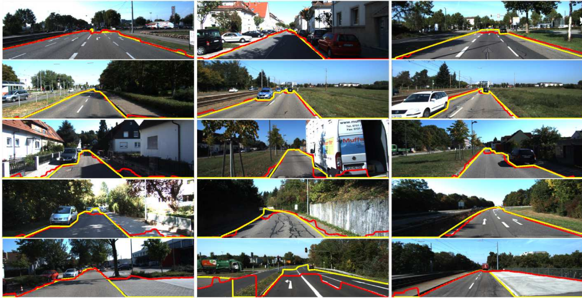
Figure 7. Example results from KITTI road dataset. The top four rows show some of the best performing scenes, demonstrating accurate results given by our approach. The last row shows worst performing scenes; failure modes are typically due to road markings and confusion between pavement and road.
