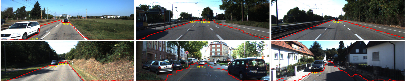
Figure 5. The red curve is the result from our model. When the parameters of the camera are known, we can estimate the distance from the obstacle to the camera (yellow text).
