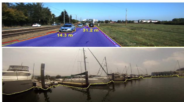
Figure 1. (Top row) An image captured from the front of a car while driving on a road. The red curve shows the ground truth free space where the car can move without colliding with other cars and obstacles. The yellow curve shows the free space estimated using our algorithm. The blue marked region is the ground truth road classification. The numbers indicate the 3D distance from the camera to the obstacle estimated by our approach. (Bottom row) An image captured from a boat. The single yellow curve represents the free space where our result and the ground truth coincide visually.
