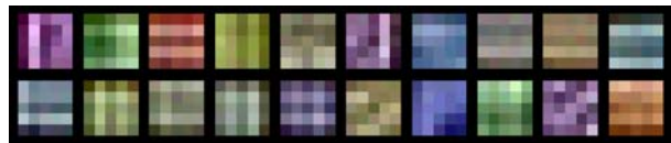
Figure 4: Visualization of the weights learned in the first tied convolution layer. Each filter has size 5 \times 5 \times 3 .
