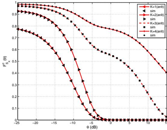
Fig. 1. Analytical (antl) and simulation (sim) results for the CCDF of  $S_K$  for various values of  $K$  with  $\Lambda = [10, 10, 0.1, 0.01]$ , and  $\{p_1 = 0.8, p_2 = 0.7, p_3 = 0.6, p_4 = 0.5\}$ .
