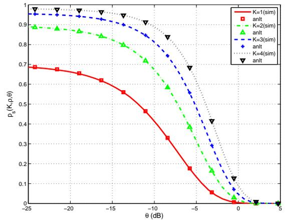
Fig. 2. The success probability for various values of  $K$  with a symmetric node geometry. Analytical (antl) results match with the simulation (sim) results. Simulation parameters are  $\rho = 10$ ,  $\eta = 3.6$ ,  $\{x_i\}_{i=1}^K = 3$ , and  $\beta_i \in \{0.7, 0.65, 0.6, 0.55\}$ .
