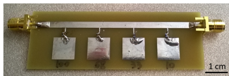
Figure 9: Fabricated capacitive sensor array on a microstrip line with connected surface mount inductors.
