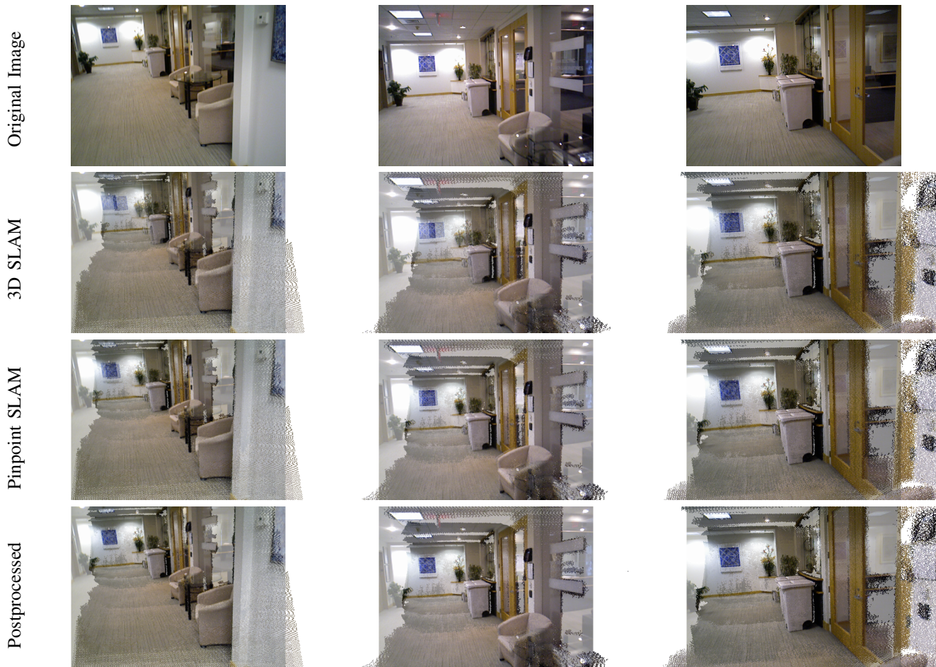
Fig. 4. Visual results on three example keyframes of the lounge sequence. Frames are overlaid on 3D reconstruction results with some transparency for better visualization. Rows show original image, 3D SLAM, pinpoint SLAM and postprocessing results from top to bottom. 3D SLAM registers the nearby regions well, but has trouble matching further points (notice the area around the frame on the wall). Pinpoint SLAM and postprocessing improve the results, producing almost perfect alignment.
