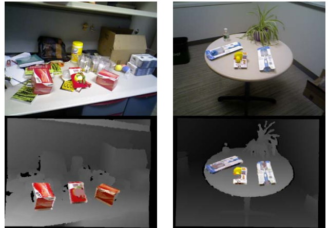
Fig. 5. Object detection results in an office sequence: input frames (top), object localization results overlaid on depth map (bottom).
