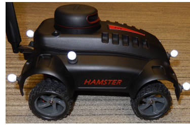
Fig. 2. The Ackermann-steered Hamster mobile robot used in the experiments. The markers (five visible in the figure) are used to track the robot via an Optitrack motion-capture system (Fig. 3).
