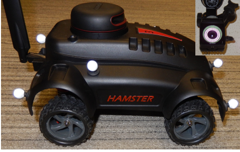
Fig. 11. The Ackermann-steered mobile robot used in the experiments. A camera from the Optitrack motion-capture system is in the top right.
