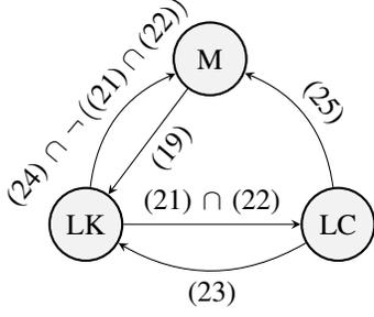
Fig. 1. Diagram showing the logic for switching between manual mode (M), lane-keeping (LK), and lane change maneuver (LC), with labels on the nodes showing requirements for transition
