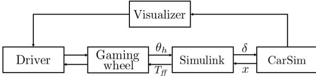
Fig. 2. Schematic of driving simulator setup
