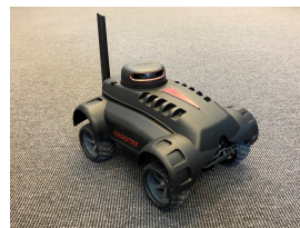
Fig. 10. The Ackermann-steered mobile robot used in the experiments.
