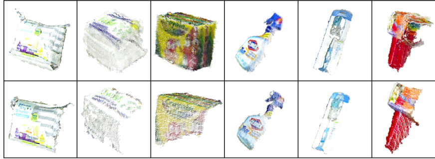
Fig. 9: Top row: Object models obtained from single object scenarios with multiple interactions. Bottom row: Object models obtained from the IP experiments with clutter. Models and experiments videos available on request.
