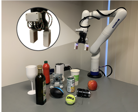
Fig. 1. Experimental setup for tactile perception. A 7-DoF (Degrees of Freedom) arm, with attached parallel jaw gripper equipped with barometric tactile sensors (zoomed-in insert).
